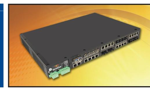
The Magnum 10KT Switch Provides Rack-mount Space Efficiency and Advanced Port Configurability for Heavy Duty Industrial Applications where Maximum Fiber Port Count and Diversity are Required.
