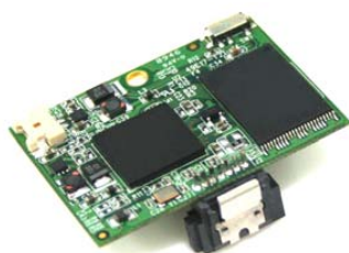
Figure 2: InnoDisk SATADOM i100 Horizontal type picture
