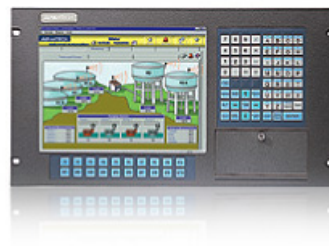
Compact Workstation with 12.1" LCD & 8 Expansion Slots
